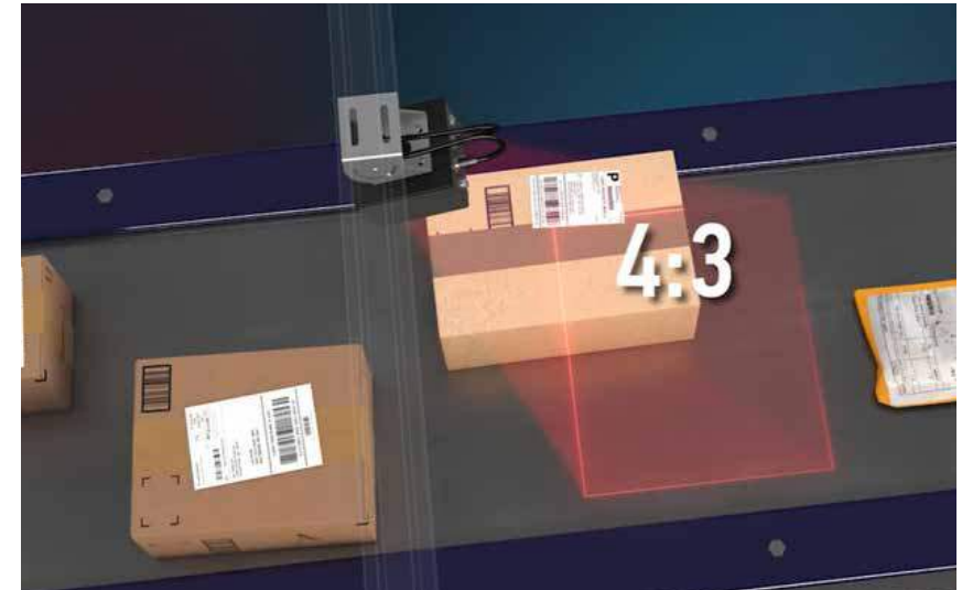
Parcels travelling on a conveyor with a 4:3 FOV barcode scanner
